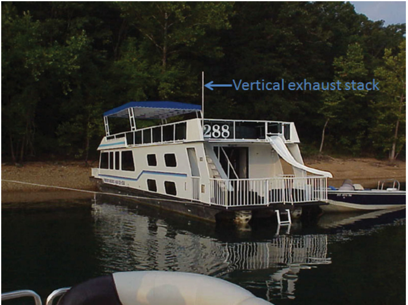
FIGURE 2. Houseboat with vertical exhaust stack.
