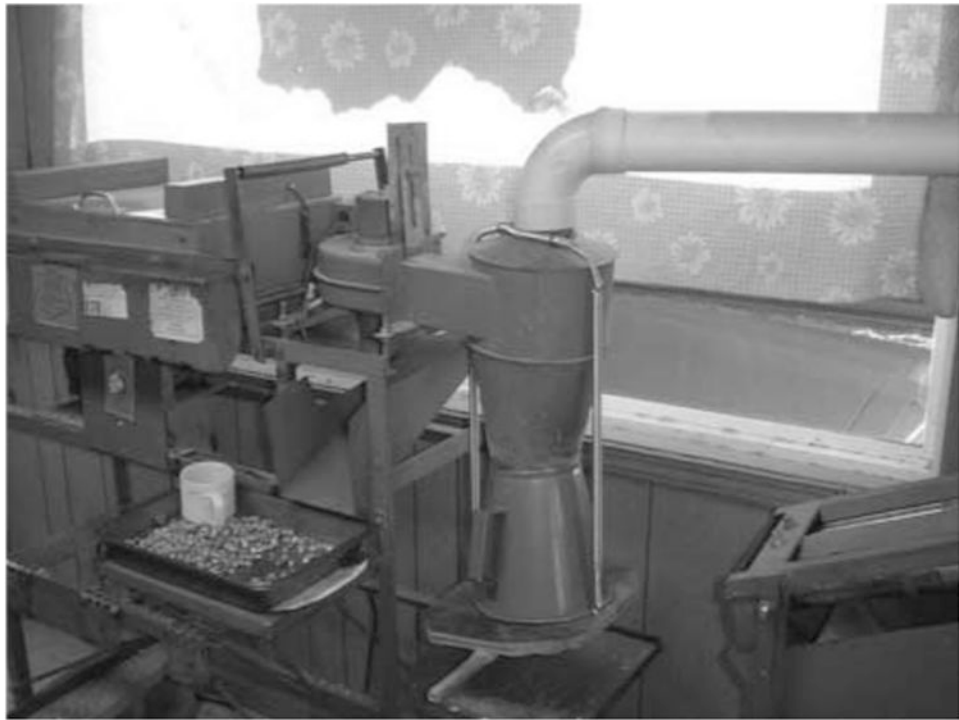
Figure 1. Peanut grading machine with retrofitted exhaust ventilation duct in 2008
