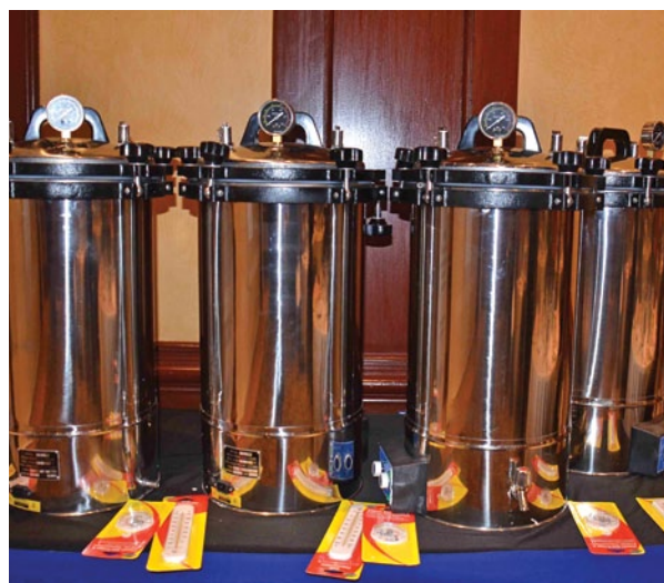
Through its cooperative agreement with the MOH, CDC provides resources like these autoclaves that sterilize laboratory infectious waste.
