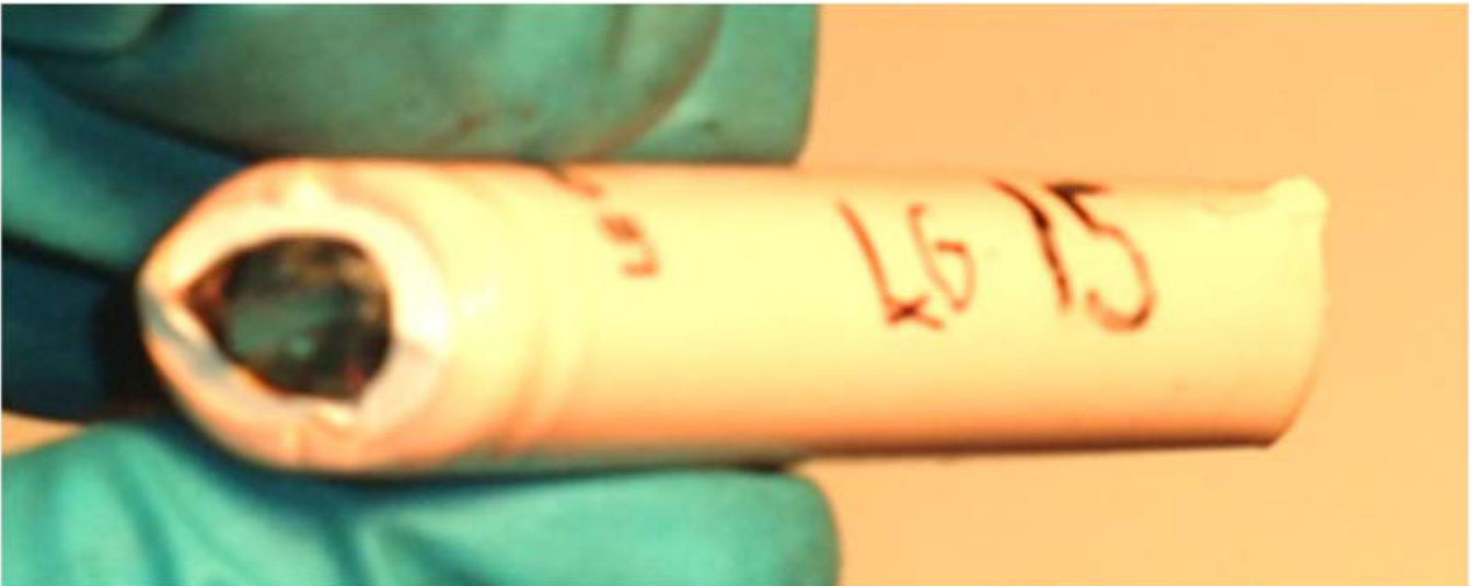
Fig. 3. Flat plate compressed the LG Chem cells about 18% without igniting 6.5% CH 4 -air.
