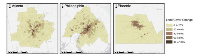
Figure 2. Percent of census tract area modified through the ALL heat management scenario. Land cover changes include the addition of new tree canopy, grass, or shrubs; conversion of roofing areas to greenroofs or high albedo materials; and the conversion of streets and other surface paving to moderate albedo materials (see Table 1). doi:10.1371/journal.pone.0100852.q002
