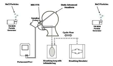
**FIGURE 1. Experimental setup for fit evaluation of the static advanced headform**Note: The headform was not enclosed in a test chamber; all test equipment was set up on a laboratory bench top.
