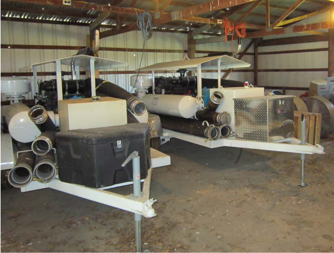
Figure A6. Portable, diesel-powered blowers for borehole air supply systems.
