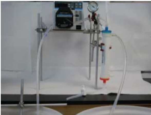
Figure 5 Dead-end ultrafiltration technique
