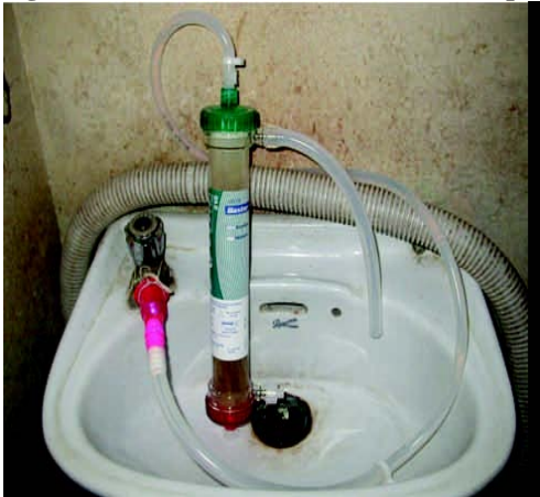
Figure 4 Dead-end ultrafiltration technique being used in the field.
