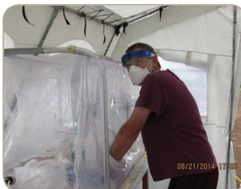
Dr. Heinz Feldman, from NIH, NIAID, Rocky Mountain lab, Hamilton, Montana, working in the glove box. The glove box was used to neutralize the virus using extraction buffer and ethanol.
