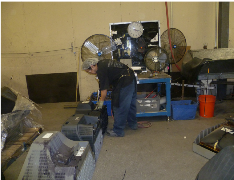
Figure 4. Employee removing CRT plastic casing with pneumatic tool. Photo by NIOSH.
