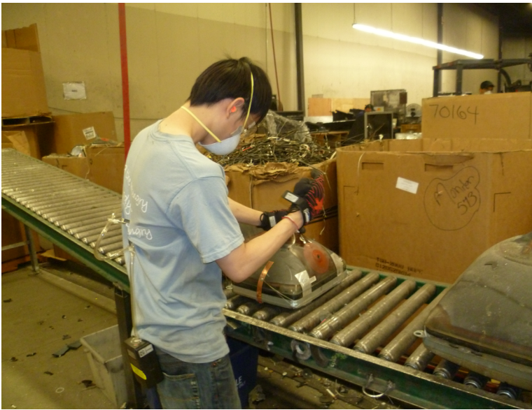
Figure 3. Employee removing wires and other circuitry before breaking of the electric gun. Photo by NIOSH.
