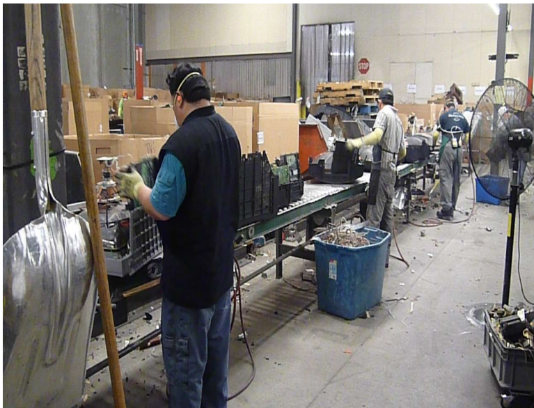
Figure 2. Employees dismantling televisions and computer monitors. Photo by NIOSH.
