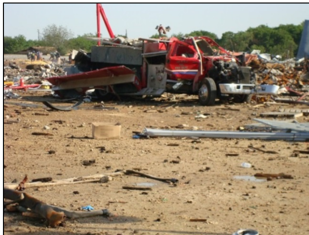
Engine 2 post explosion. Note that it is believed the force of the explosion moved the engine from its original location and orientation at the time of the blast.
