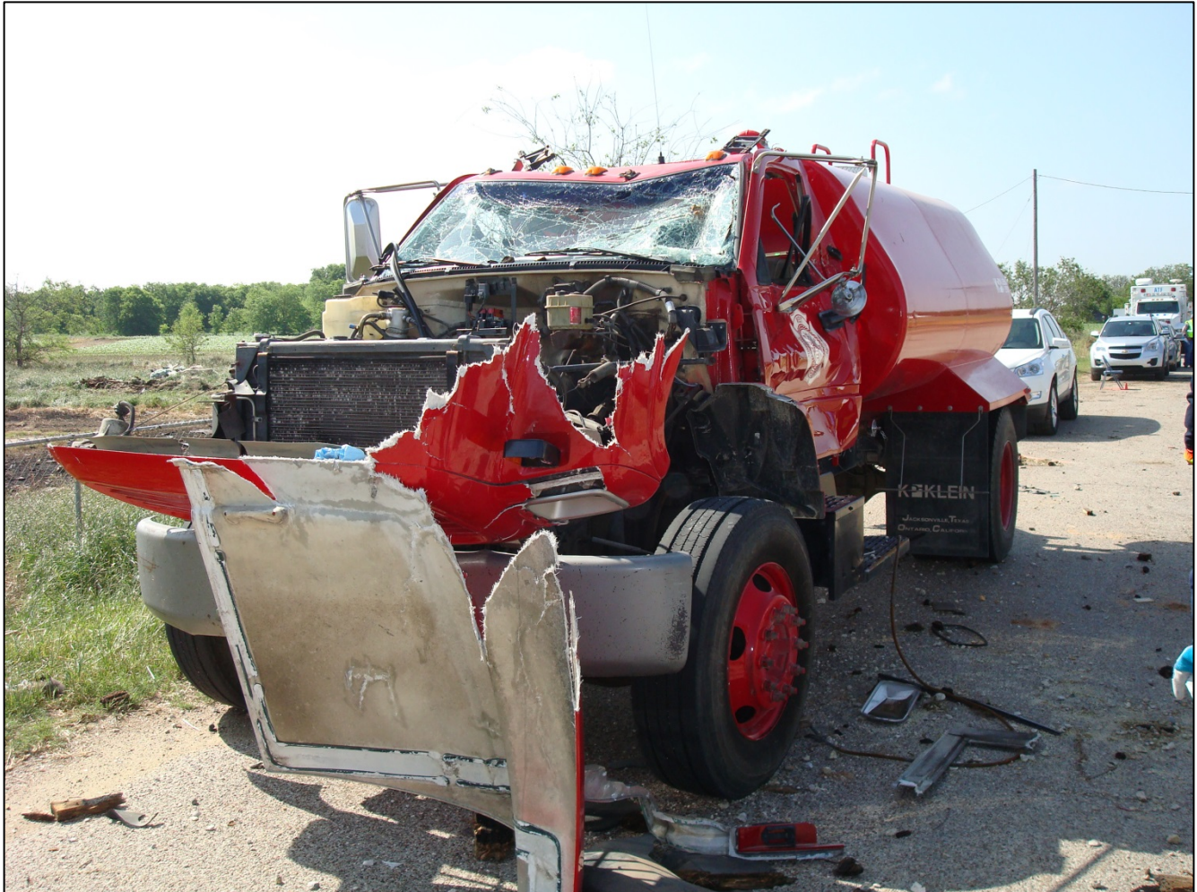
Photo 7. Damage to Tanker F-7. Tanker is shown in the same location on county road east of fertilizer plant as it was at the time of the explosion several hundred feet from the center of the explosion.
