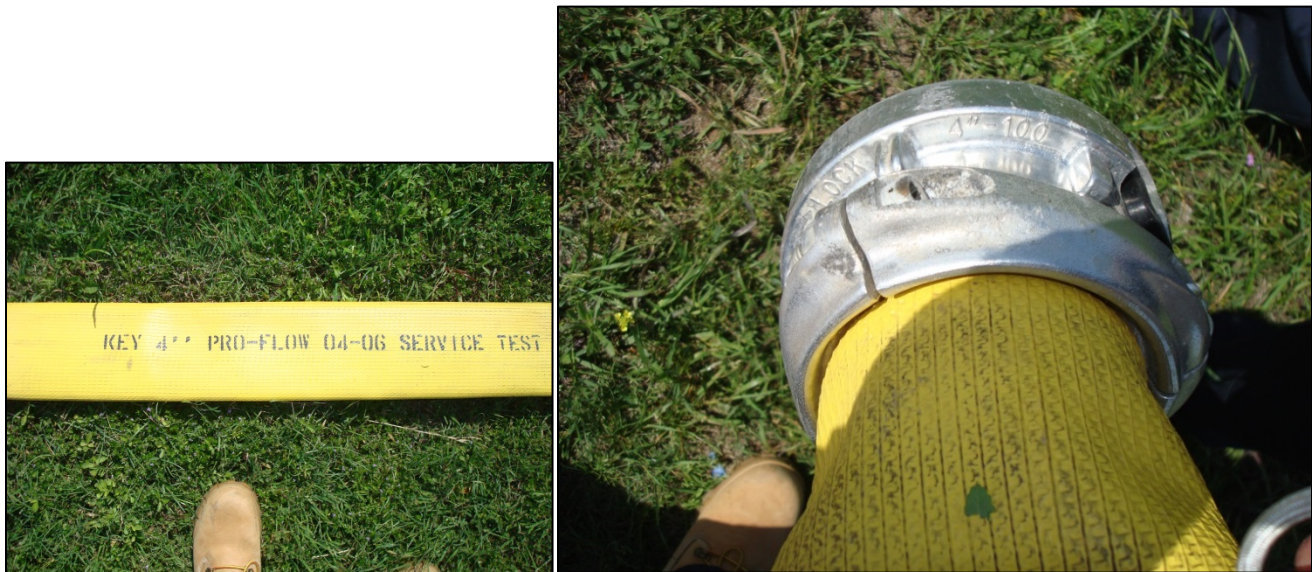
Photo 5 and Photo 6. Close-up views of 4-inch supply line (on left) and coupler (on right). (Photos taken by NIOSH investigators.)
