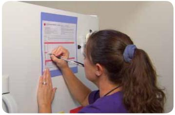
The data logger's active digital display should be attached to the outside of unit to allow reading temperatures without opening the door and disturbing the probe. Set data loggers to measure temperatures at regular intervals.
