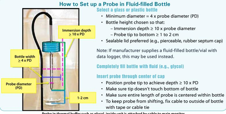
Probe in thermal buffer such as glycol, inside unit is attached by cable to main monitor
