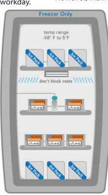
Place frozen coolant packs along walls, back, and bottom of freezer, and inside door racks.
