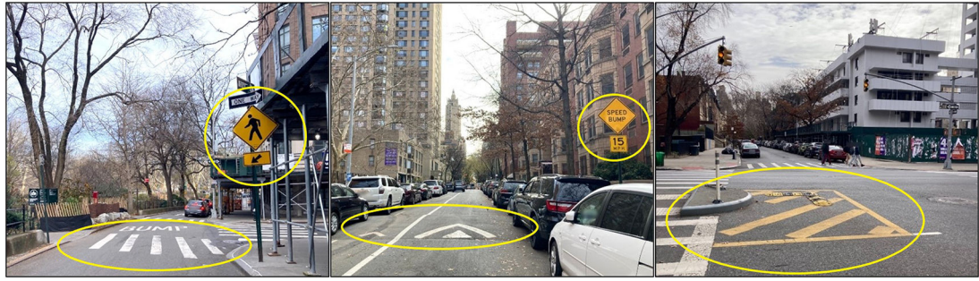
Figure 1. Example images of physical environmental roadway interventions in New York City from left to right: enhanced crossing, speed hump, turn traffic calming treatment.
