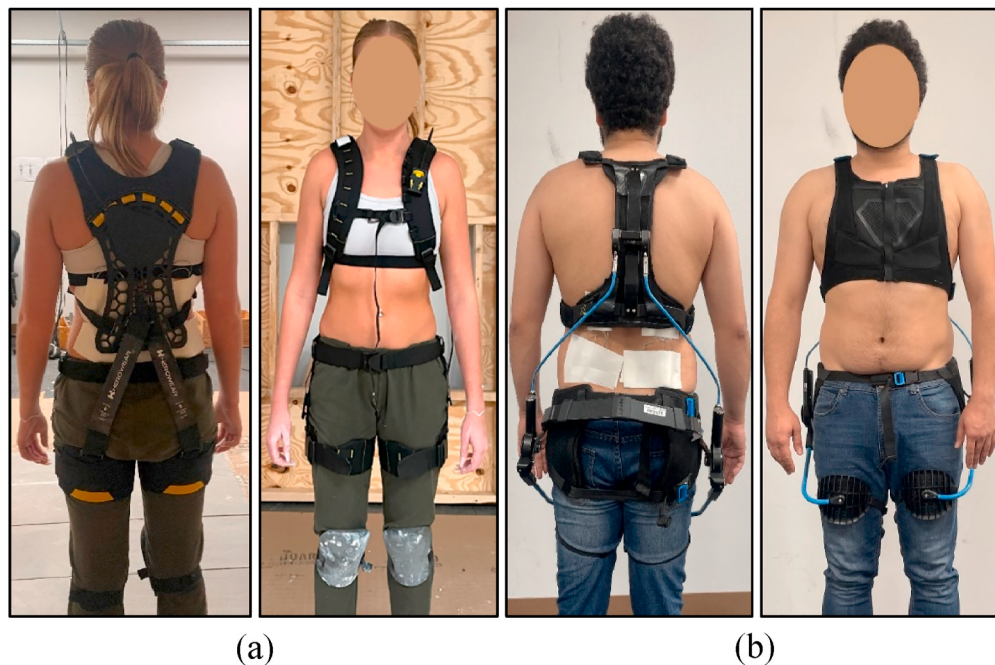
Fig. 2. Participants wearing (a) HeroWear Apex (HW) and (b) Laevo Flex (LV) exoskeletons, a demonstration of how both BSEs fit the body on the dorsal and ventral sides.
