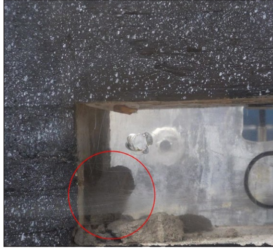
Figure 10. Failed brow observed during Test 3
