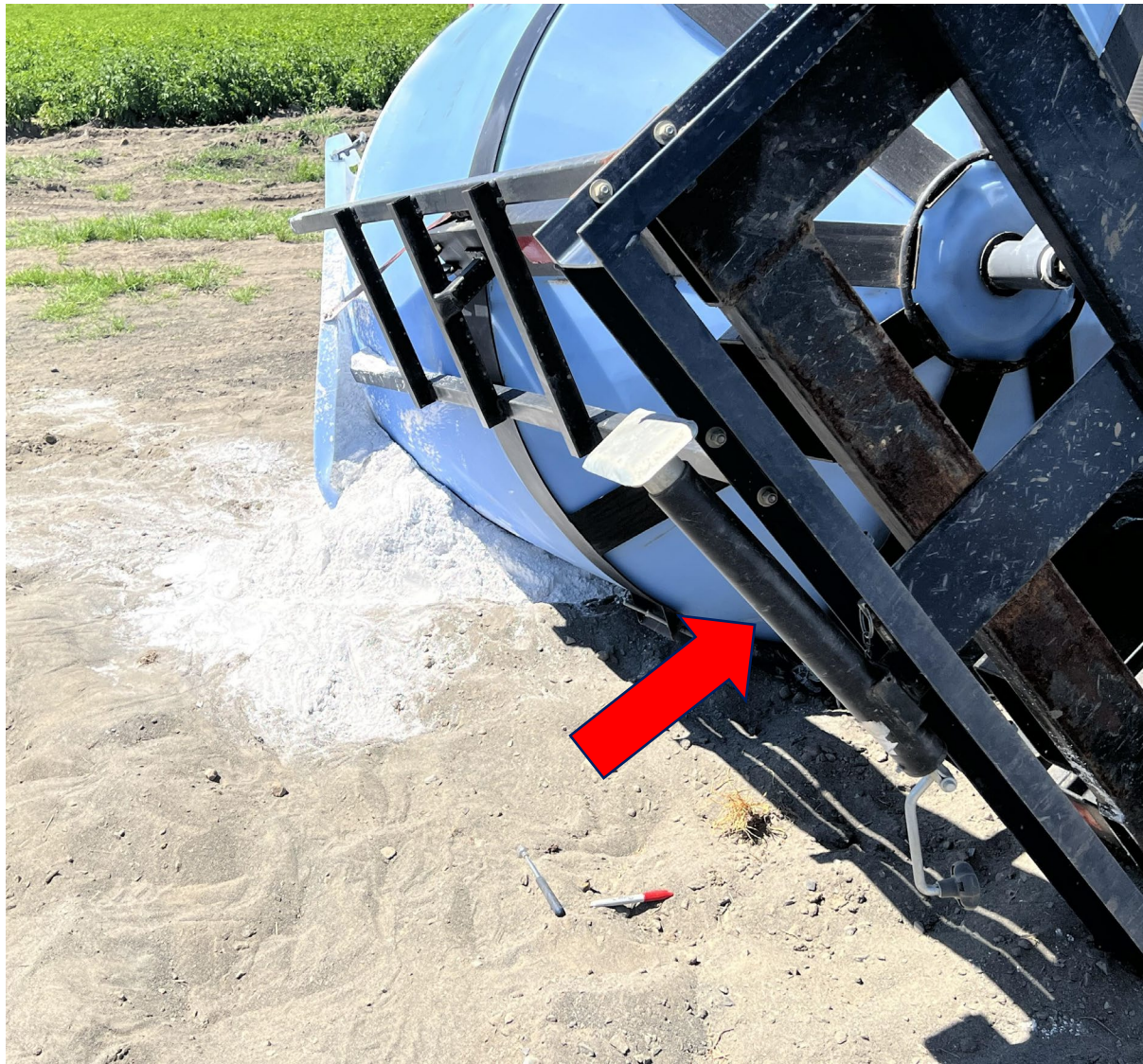
Image 3. Rear view of trailer and tank resting on soft sandy ground. Arrow points to unused jack attached to rear of trailer frame.
