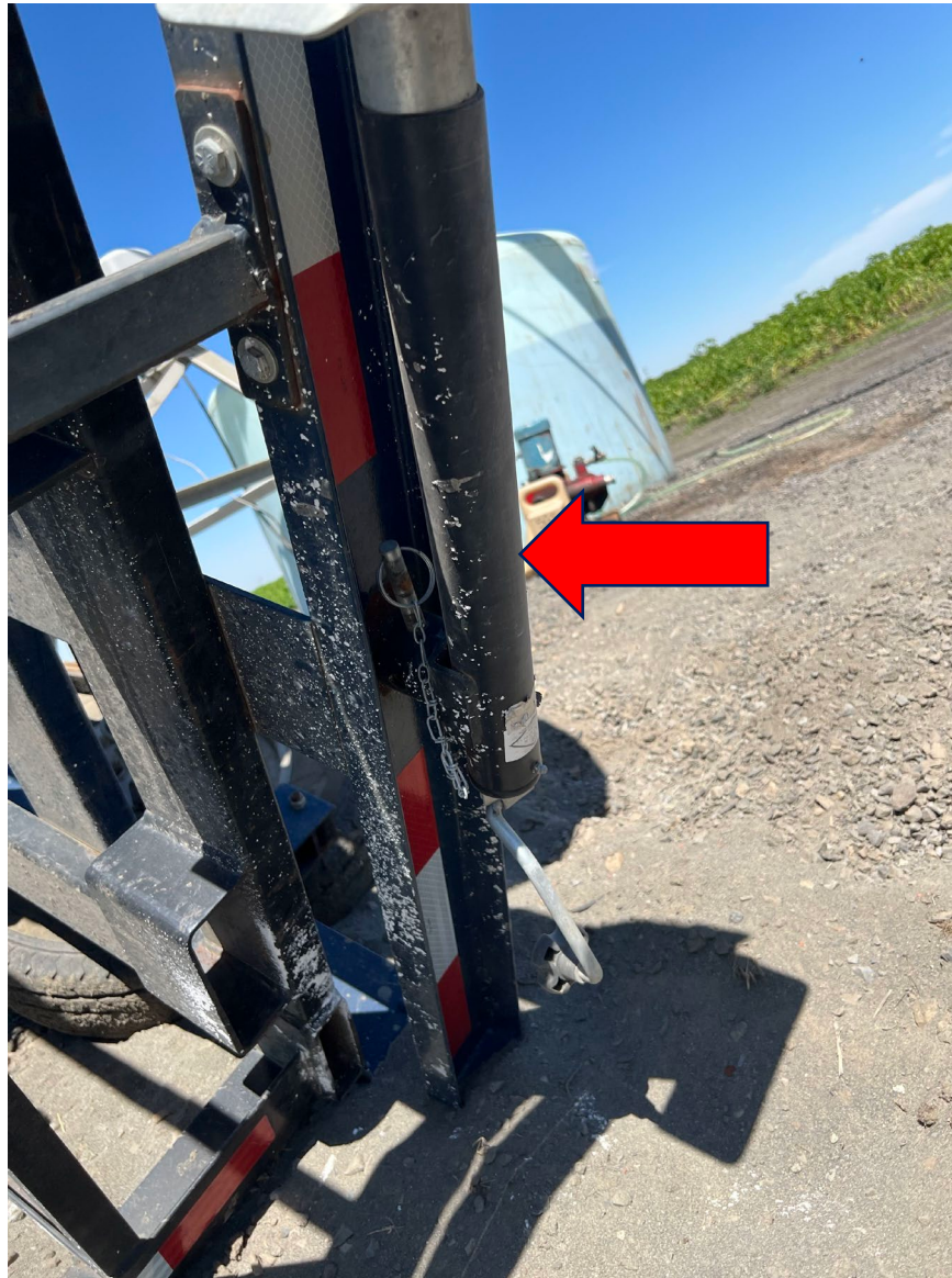
Image 4. Close-up of unused rear parking jack on trailer.
