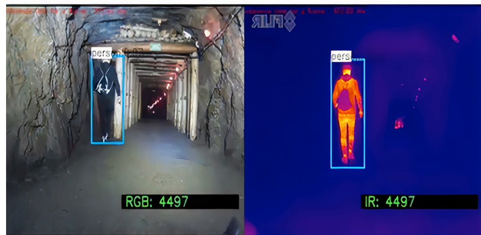
Figure 4. Thermal imagery using YOLO algorithm for underground pedestrian detection [42].
