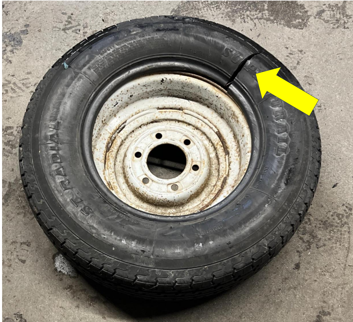
Image 3. Ruptured tire after explosion.
