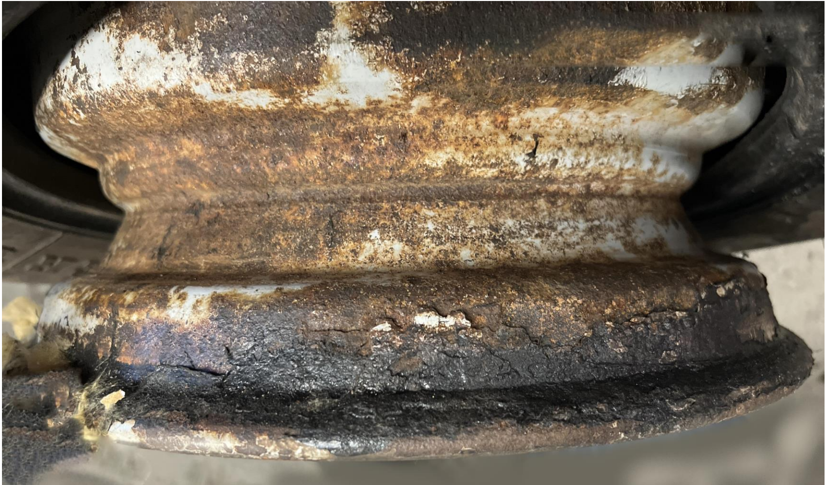
Image 4. Corrosion on tire rim and bead seat.
