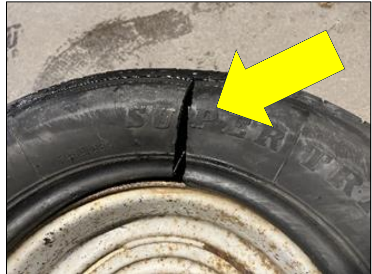
Image 1. Ruptured sidewall on tire that exploded.
