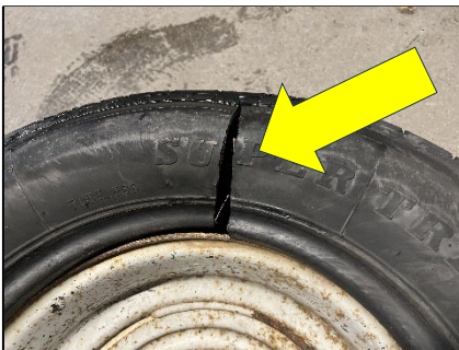
Ruptured sidewall on tire that exploded.
