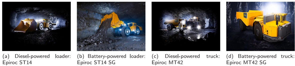
Fig. 2. Diesel-powered loaders and trucks versus their battery equivalent (Epiroc, 2024). These are for visual purposes only.
