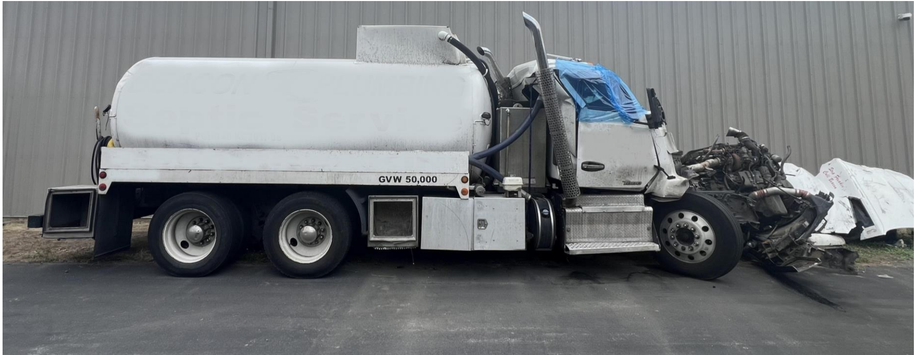
Image 6. Tanker truck with collision damage.
