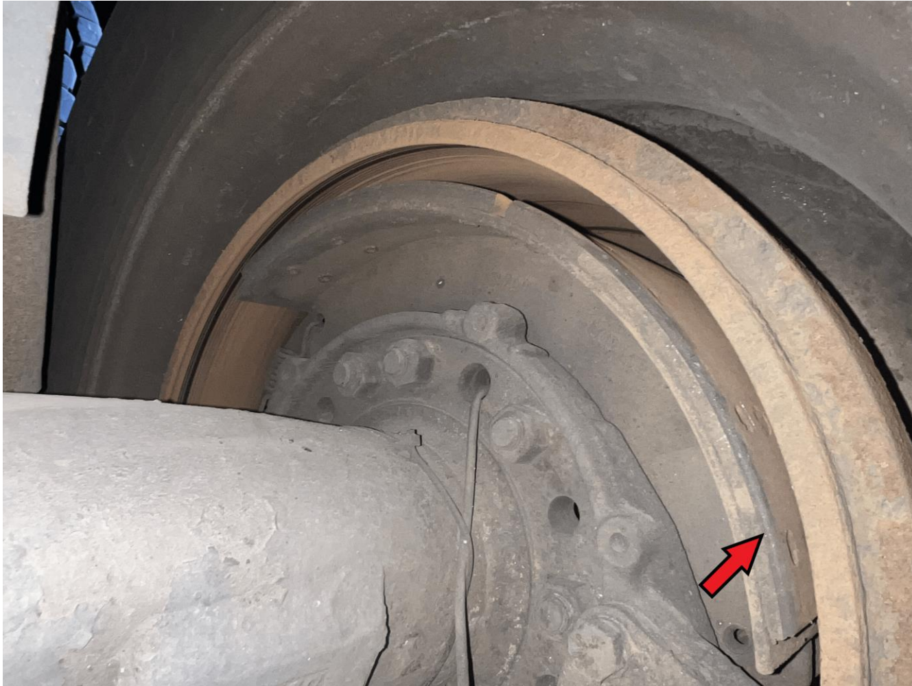
Image 8. Upper brake shoes not in contact with drum while emergency brake is engaged.
