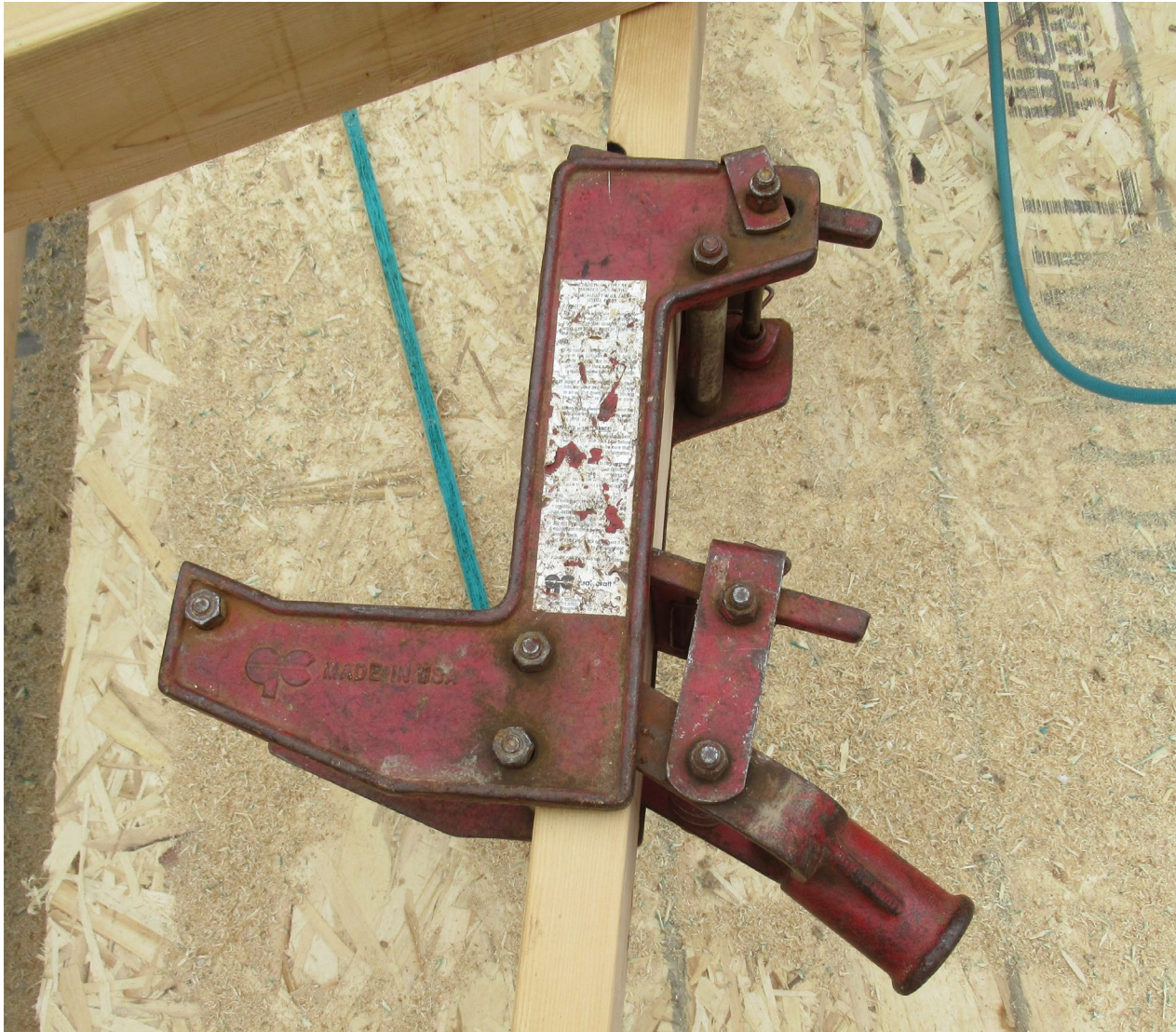
Image 4. Wall jack attached to wood post.
