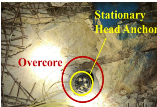
Fig. 12 MPBX A0X3 installed in the borehole, recessed in overcore
