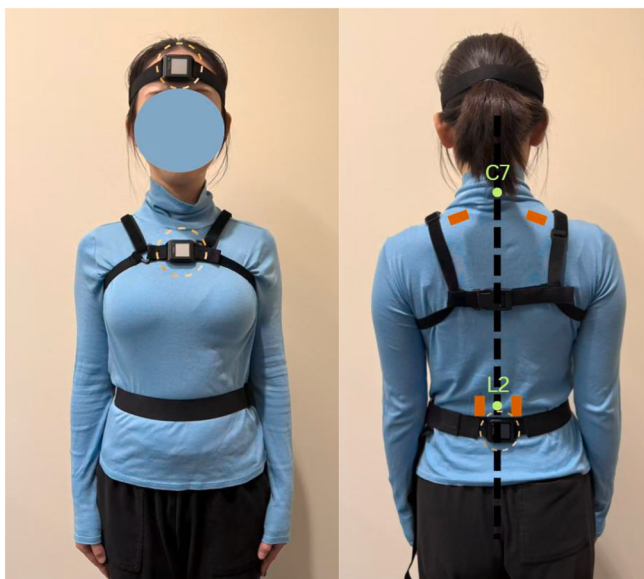
Fig. 2. Locations of EMG and APDM IMU sensors. The C7 and L2 vertebrae served as spinal reference points. Orange rectangles indicate EMG sensor positions, which were placed directly on the skin beneath the clothing. The straps and OPAL units (marked with yellow dashed circles) represent the IMU sensors.
