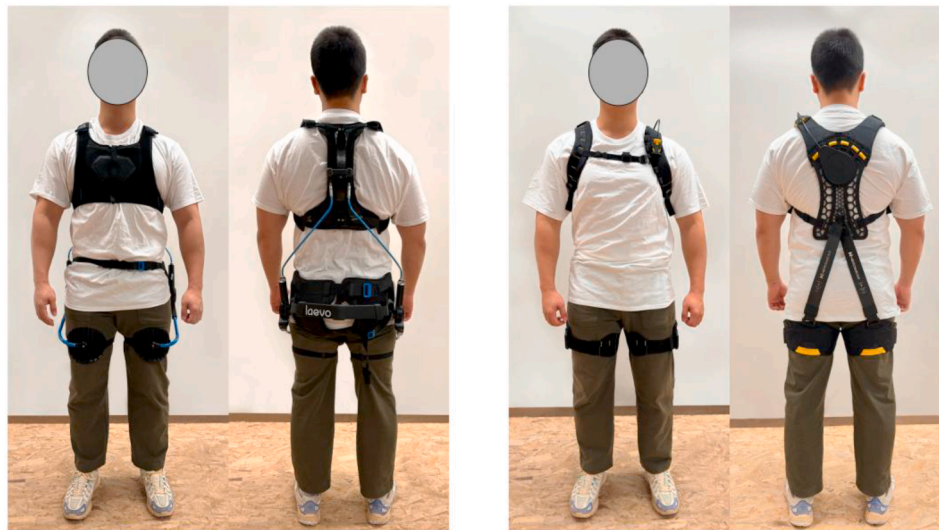
Fig. 2. The two back-support exoskeletons (BSEs) included in the study: (Left) a rigid BSE, Laevo FLEX and (Right) a soft BSE, HeroWear Apex 2.
