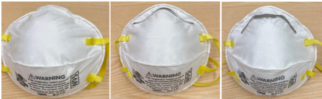
Figure 1. N95 FFRs illustrate three noseclip conditions: (left) without a noseclip, (middle) with a conventional adjustable metal noseclip, and (right) with an M-shaped adjustable metal noseclip.
