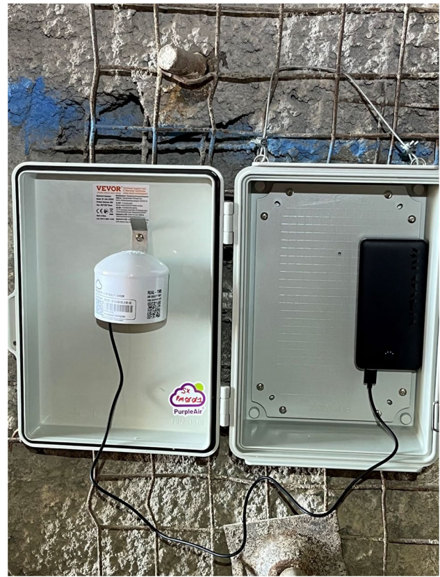
Fig. 2 PurpleAir Classic air quality monitor installed in the underground mining facility connected to a rechargeable 20 Ah battery
