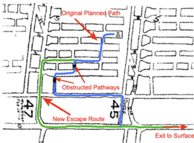
Fig. 4. Post-disaster escape routing: disaster-induced blockages invalidate the original evacuation plan, necessitating a revised path that safely guides miners toward the surface [9].
