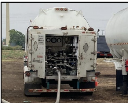
Control cabinet with transfer hose at back of transport trailer.
