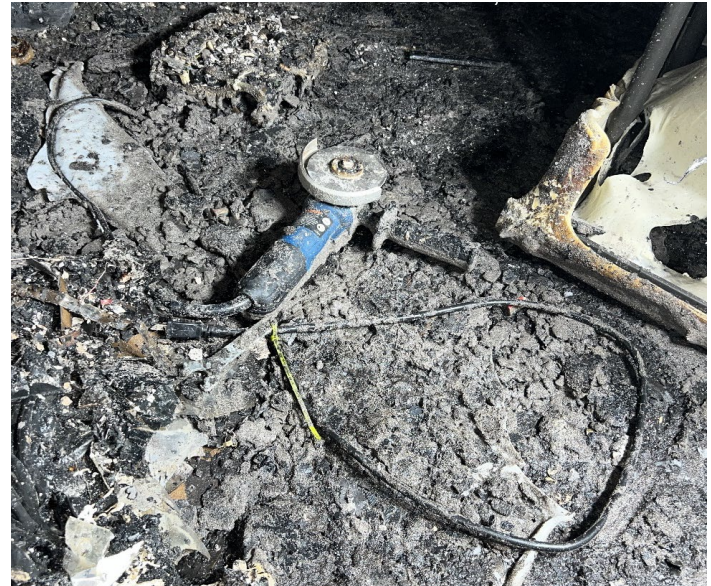
Image 1. Angle grinder where fire started.
