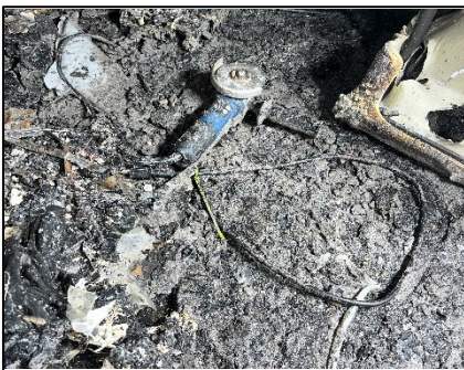
Angle grinder where fire started.
