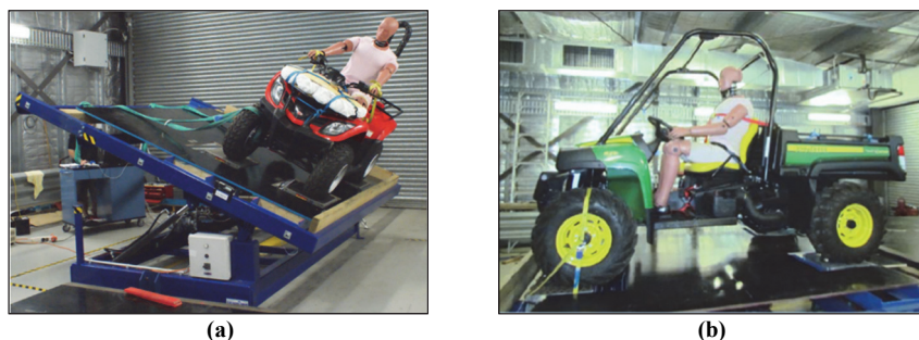
Figure 1. (a) Quad bike with rollbar and (b) SSV, both fitted with an anthropomorphic test device (ATD), subjected to lateral, rear, and forward pitch tests (Grzebieta et al., 2015a).
