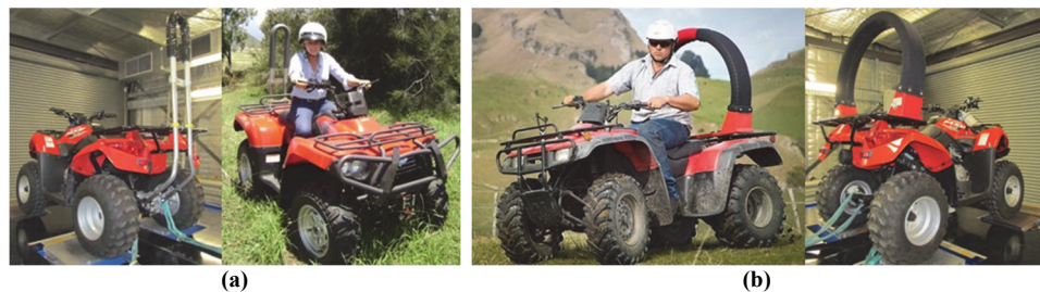
Figure 2. Operator Protective Devices (OPDs): (a) Quadbar and (b) Lifeguard (Grzebieta et al., 2017).
