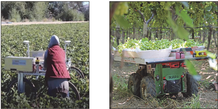
Figure 3. Examples of collaborative robots developed in academia: (left) "FRAIL-bots," get the full strawberry trays from pickers (Peng et al., 2021, 2022), and (right) a commercial collaborative robot, Burro 9 (www.burro.ai).
