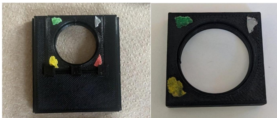
Figure 2. 3-D printed 25 mm cassette holder (left) shown with the square cassette (right).
