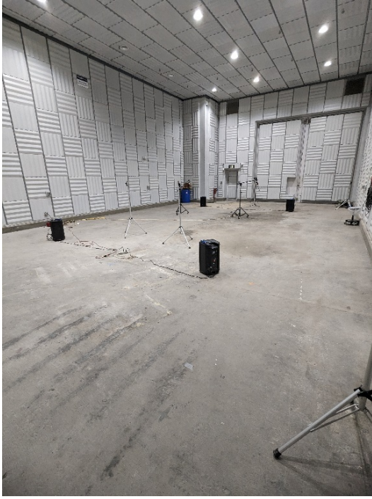
Fig. 1. The 16.6 m x 9.9 m x 6.4 m NIOSH Hemi-anechoic Chamber (HAC).
