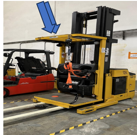
Exhibit 3: The order picker forklift involved in the incident. The arrow indicates where the self-retracting lanyard connected to the body harness was hooked to the forklift. Photo courtesy of CA/FACE program.
