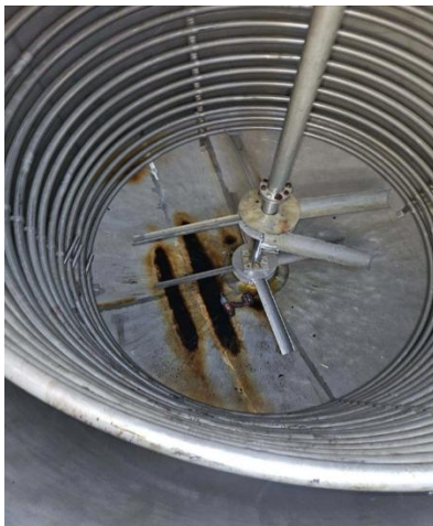
Exhibit 2: Blades inside the motor oil tank. Photo courtesy of the oil company.
