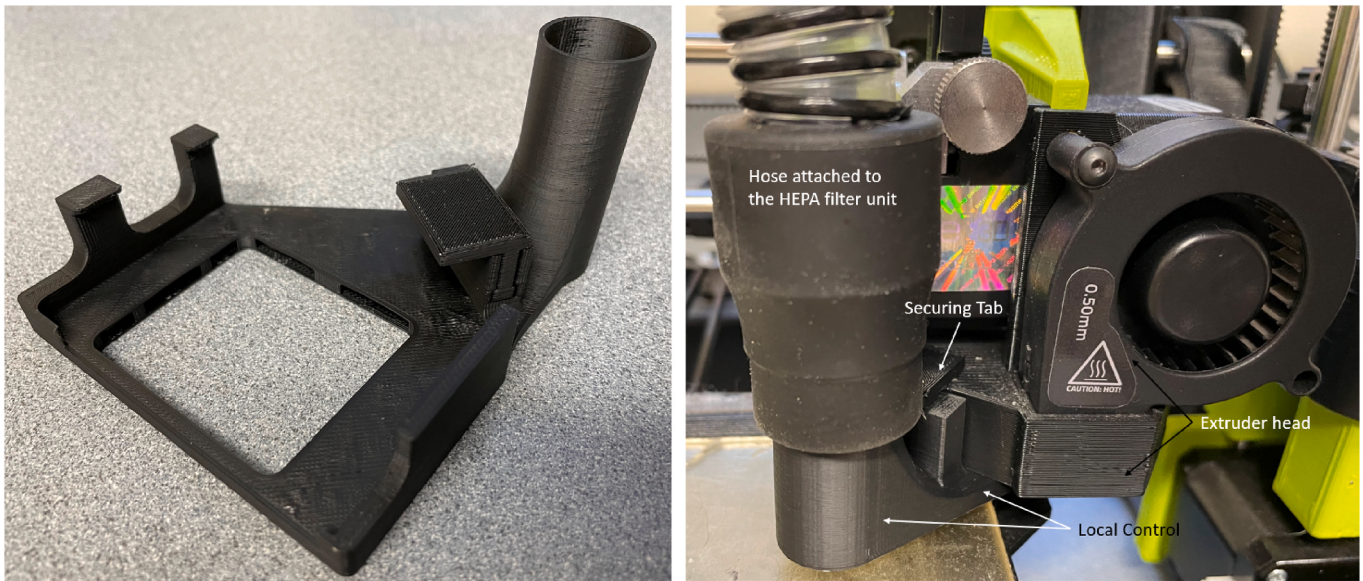
Fig. 6. Printer 2 LEV Control B with tab inserted (left) and control attached to printer extruder head (right). Photos by NIOSH.
