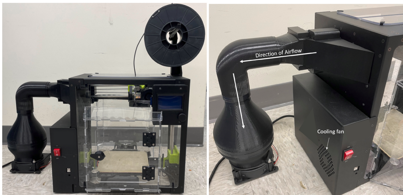
Fig. 7. Printer 2 outfitted with commercially available enclosure and HEPA filtration unit. Image on right shows the cooling fan vent linked with particle reduction issues discussed below. Photos by NIOSH.
