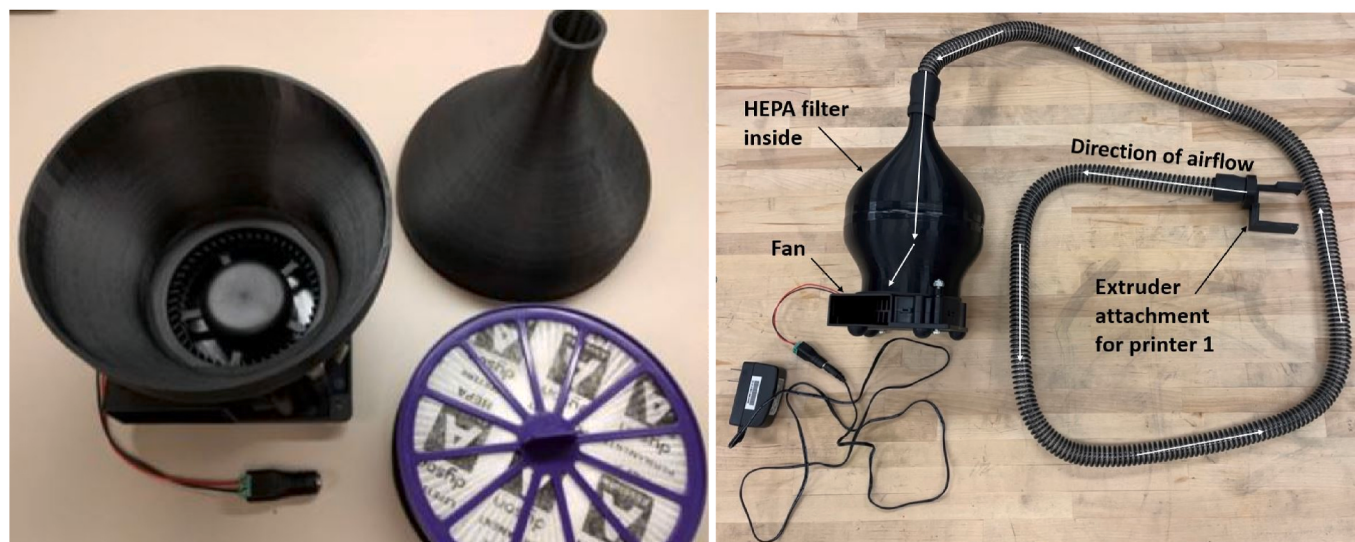
Fig. 4. Low-cost air cleaner assembly connected to a 3D printer ventilation control piece. The HEPA filter is 14 cm (5.5 in) in diameter and 2.5 cm (1 in) in thickness. Hose is shown with Control A attached.
