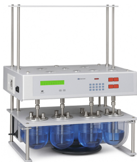
Figure A1. Varian VK 7000 dissolution apparatus.
