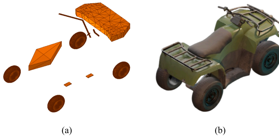
Fig. 6. 3-D representation of ATV mock-ups. (a) Example of a 3-D ATV mock-up used for the virtual simulations in SAMMIE CAD (Araujo et al., 2022) (b) Fully assembled model – for visualization purposes only.
