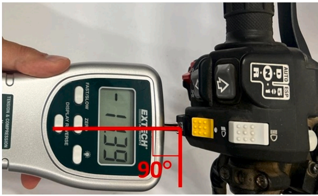
Fig. 2. A handheld force gauge is used to measure the forces that push the ignition switch on the ATV handlebar. The force gauge probe is held perpendicular to the bottom's surface.
