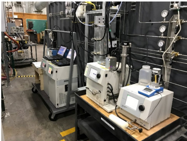
Fig. 8 The aerosol instrumentation (two FMPSs and the SMPS) outside of the test chamber
