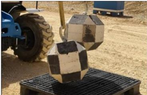
Figure 3. Rhombicuboctahedron synthetic rock (from McNabb et al., 2025 (in review)).
