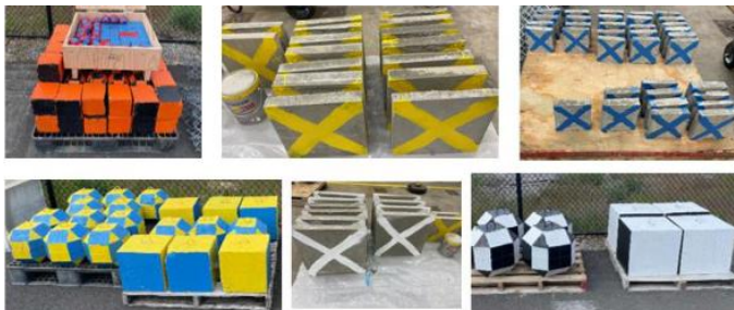
Figure 1. Different rock shapes and sizes tested in the Highwall Safety Project (from Warren et al., 2024).
