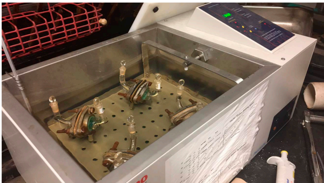
Figure 1. The permeation cell setup in the thermostatted shaking water bath at zero permeation time [29].
