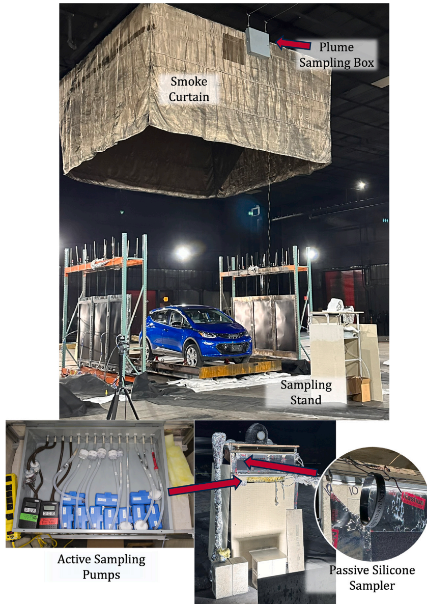
Fig. 1. Top: Overview of the experiment setup. Sampling stations were located in front of the vehicle, behind the vehicle, and above the vehicle near the ceiling. Left, bottom: exposure sampling boxes with personal air pumps where sampling media were connected to ceramic ports that extended 1.5 cm outside of the sampling box. Center, bottom: Test stands were positioned 3.0 m from the front bumper (as shown) and 4.5 m from the rear bumper of the vehicle (not visible). Right, bottom: Passive silicone samplers were placed at each sampling position.
