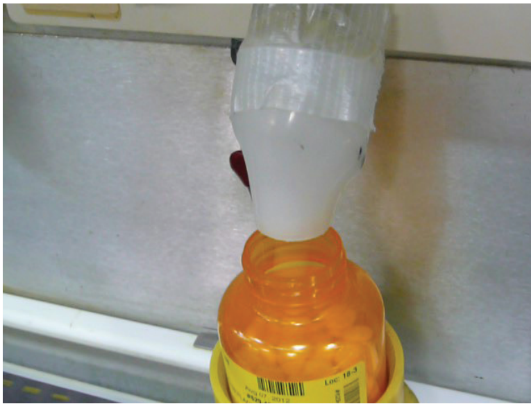
Figure 2. Baker machine nozzle where pharmaceuticals were dispensed into prescription bottles. Photo by NIOSH.
