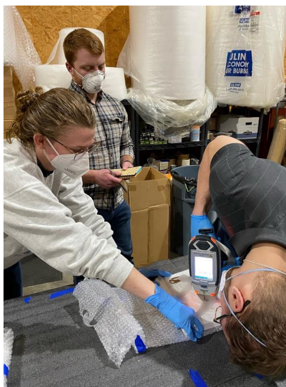
Fig. 2. Students conducting XRF testing on seized items.
