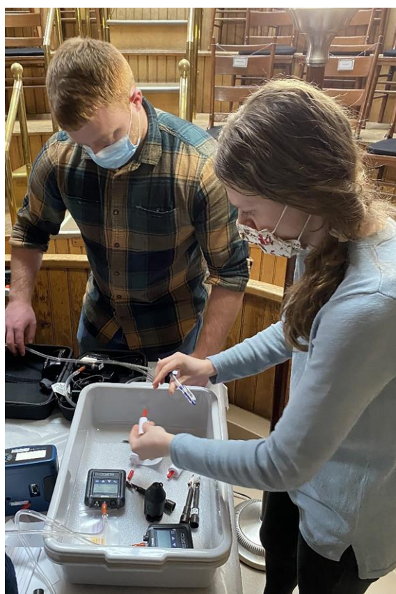
Fig. 1. Students calibrating sampling pumps for formaldehyde testing.
