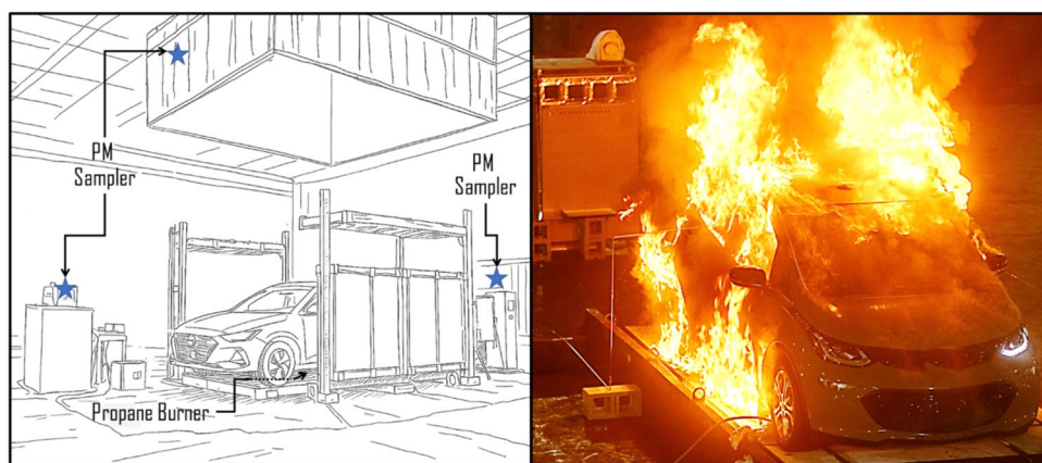
Fig. 1 Schematic of full-scale EV and ICEV fire testing (left) and one of the vehicles during the fire event (right)
