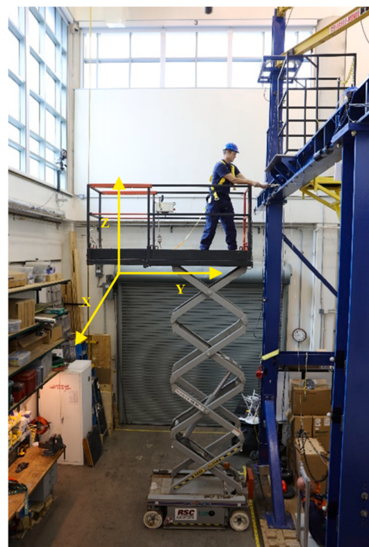
Fig. 1. Dynamic motion data of a scissor lift were collected in the high bay lab of NIOSH.
