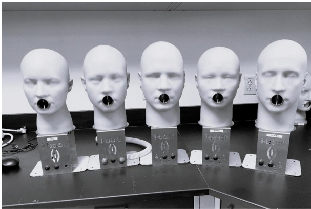
Figure 1. The complete set of ISO StAHs used for testing (five sizes from left to right: small, medium, large, short-wide, long-narrow).
