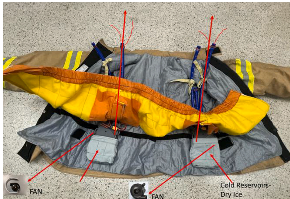
Fig. 1. The LION Cooling System coat, which used carbon nanotube-based fabric with two pouches and a fan to cool the firefighter. The arrows identify the location of the pouches which can take dry ice.
